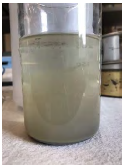
Figure 4. The clay suspension in deionized water after two weeks
