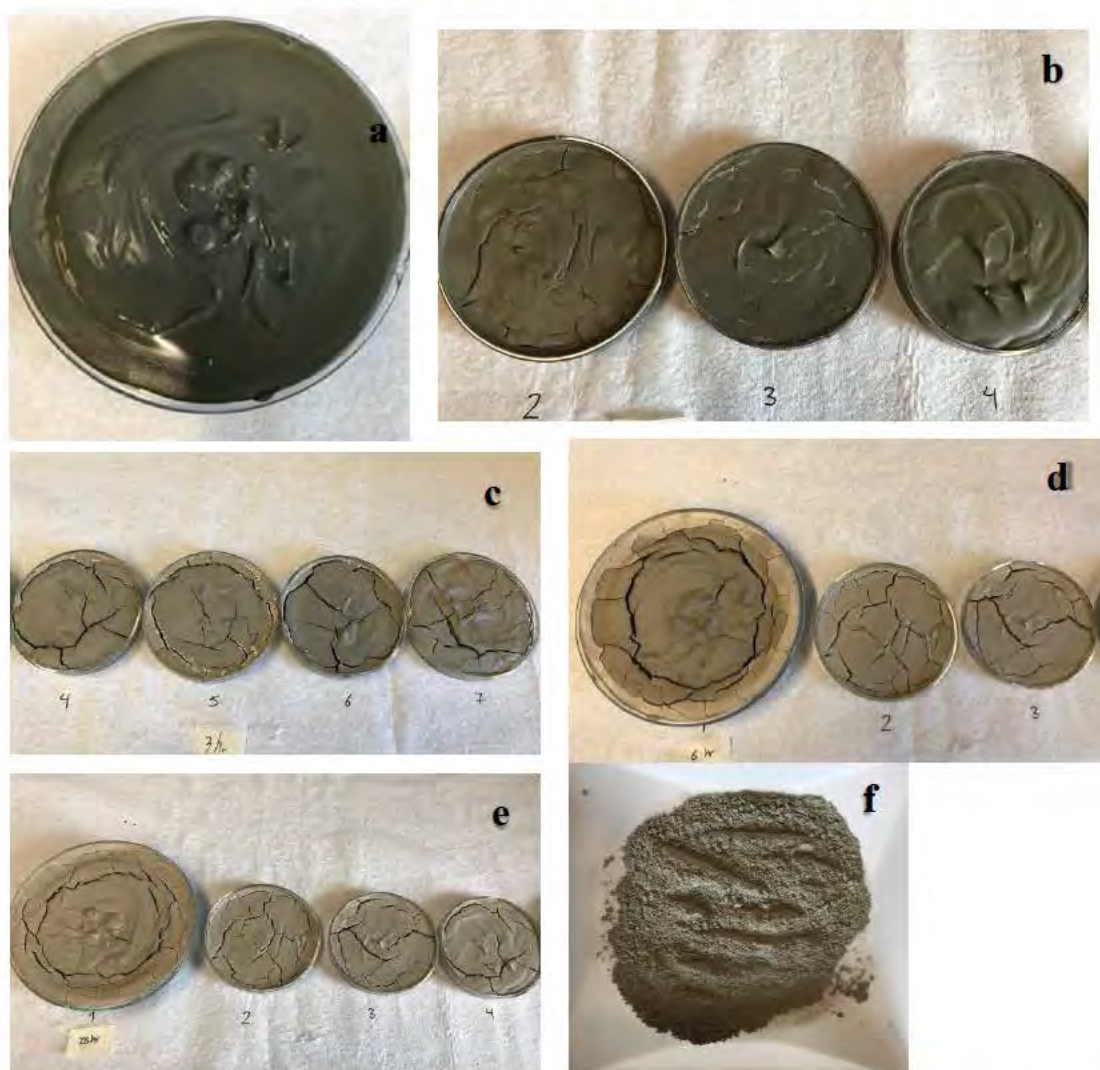
Figure 2. Clay samples in the course of drying: a) 30 min, b) 1 h, c) 3 h, d) 6 h, e) between 20 and 40 h, and f) dried clay
