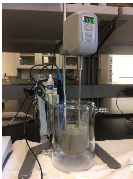
Figure 6. Leaching experimental setup
